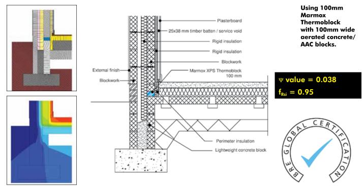
**Typical Specification:** A single course of Marmox Thermoblock: 600mm(l) x 100/140/215mm(w) x 65mm(ht) is the starter course for the inner leaf of the wall in place of the bottom row of blocks. Thermoblock is fixed to the floor with normal mortar which is also used to lay subsequent courses of bricks/blocks on top. If using lightweight blocks, this initial layer of mortar should be at least 15mm.
