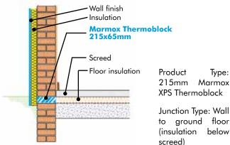
Junction Type: Wall to ground floor (insulation below
