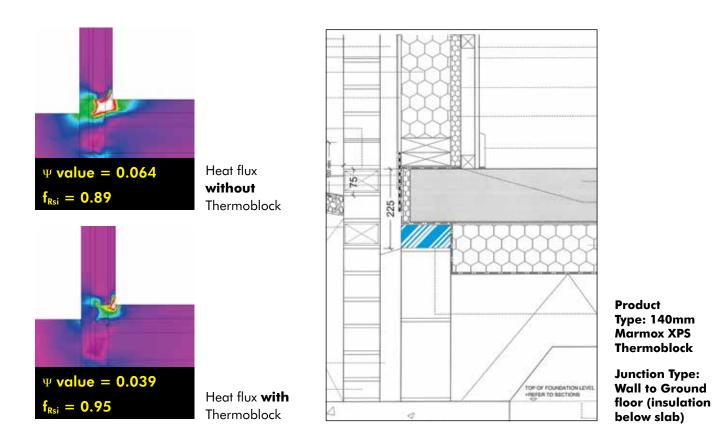
**Specification:** A single course of Marmox Thermoblock: 600mm(I) x 100/140/215mm(w) x 65mm(ht) is fixed using normal mortar on to top of the foundation blocks (inner leaf) directly underneath the load bearing concrete slab on which the timber frame is fixed.
