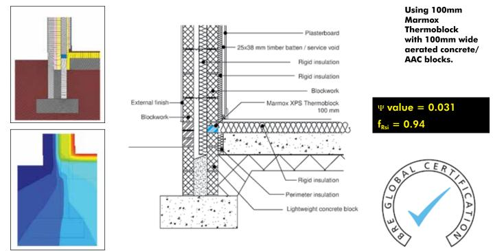
Typical Specification: A single course of Marmox Thermoblock: 600mm(l) x 100/140/215mm(w) x 65mm(ht) is the starter course for the inner leaf of the wall in place of the bottom row of blocks. Thermoblock is fixed to the floor with normal mortar which is also used to lay subsequent courses of bricks/blocks on top. If using lightweight blocks, this initial layer of mortar should be at least 15mm.
